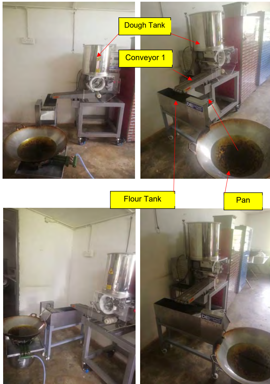
Figure 4: Actual Delivered Automated Kuih Kasturi Machine
